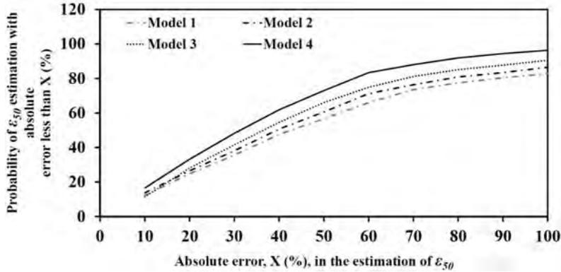
Figure 4: Probability of  $\varepsilon_{50}$  estimation with absolute error less than a given error,  $x$  (%)
