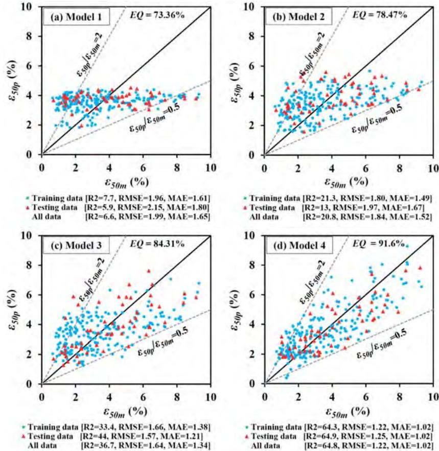
Figure 3: Predicted versus measured  $\varepsilon_{50}$  values for proposed EPR-based models
