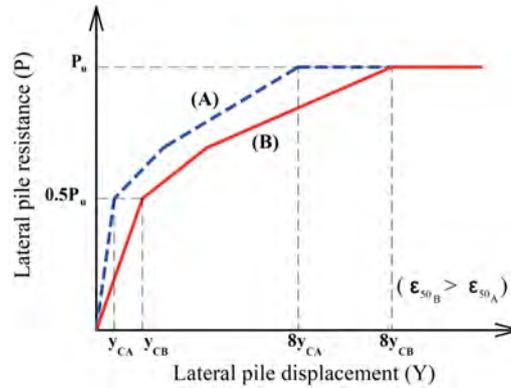
Figure 1: Typical p-y curves for pile in cohesive soil under static loading
