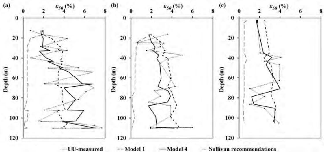
Figure 8: Profiles of predicted and measured  $\epsilon_{50}$  values in site 1 from (a) borehole 1, (b) borehole 2, and (c) borehole 3
