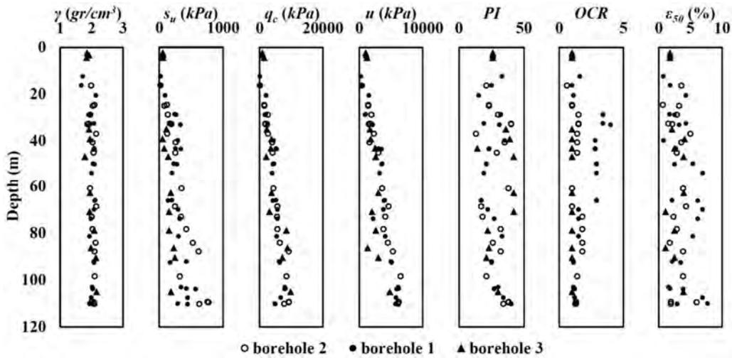
Figure 7: Geotechnical characteristics of soil in the boreholes of site 1
