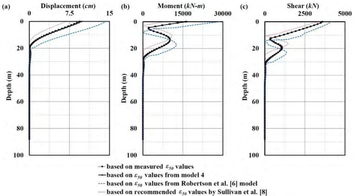
Figure 9: Numerical analysis results of lateral response of typical pile-soil system
